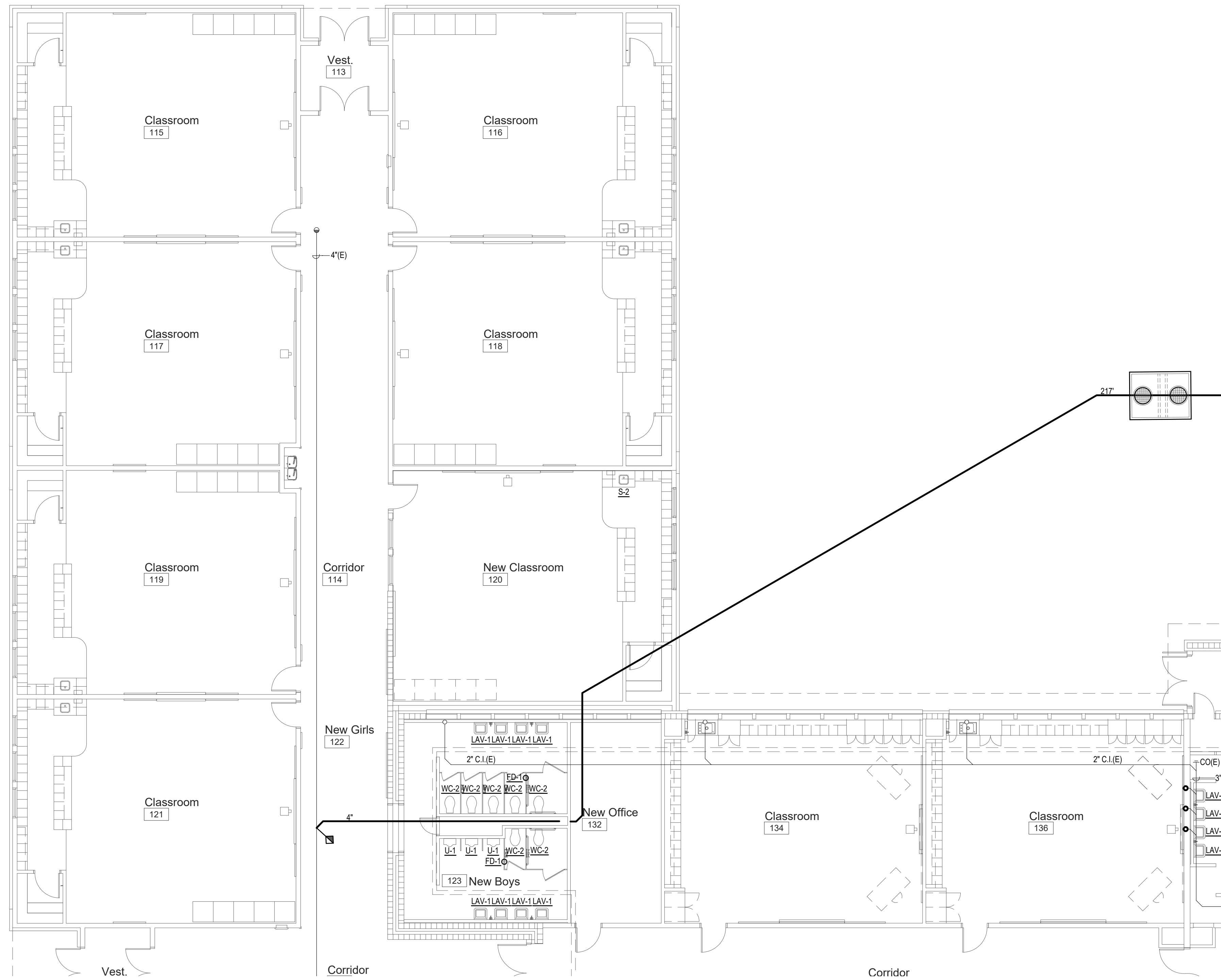
1 Plumbing New Work Plan - Area 'A' Scale: 1/8" = 1'-0"
